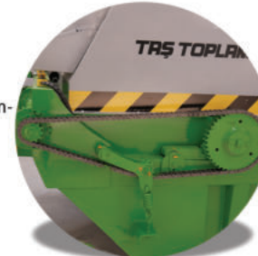
-Automatic chain tensioning system-
